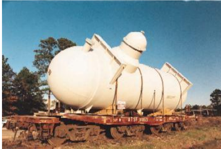
High pressure separator for a refinery in south Louisiana. Shell Plate 4.375" thick, ASME Section VIII, Div.2 with 13" wall thickness sump. Shipment by rail in early 1993.
