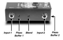
input impedance to 10meg ohms. This ensures the piezo pickup "sees" the optimum input impedance for signal transfer which will result in better tone. To activate the piezo buffer use a tweaker (small screwdriver) to push in the recessed PZB switch. There is a separate PZB switch for each input channel.
