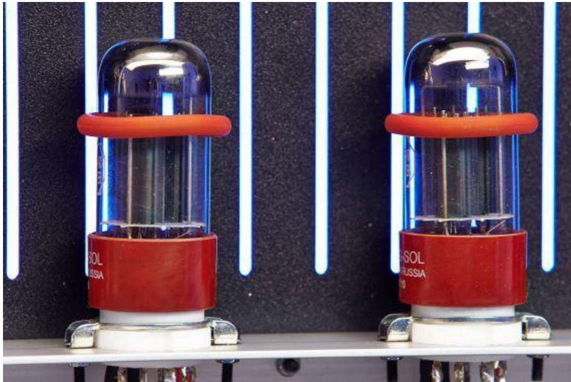
A RARE SIGHT IN A PREAMPLIFIER: VALVET EMPLOYS IN THE L2 6SN7 TWIN TRIODES – A TUNING DREAM FOR EXPERIENCED TUBE-ROLLERS
